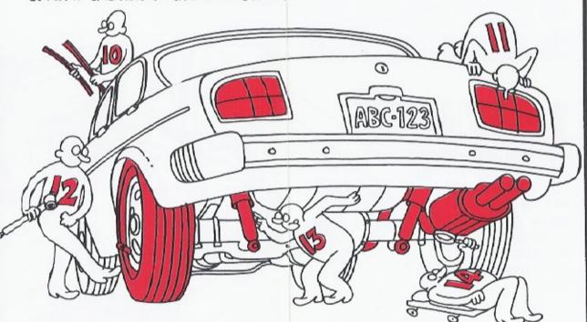
KEEP TIRES INFLATED TO RECOMMENDED PRESSURE (IT HELPS TO OWN YOUR OWN GAUGE). CHECK FOR CUTS, BULGES AND EXCESSIVE TREAD WEAR. UNEVEN WEAR INDICATES MISALIGNMENT OR OUT-OF-BALANCE.
